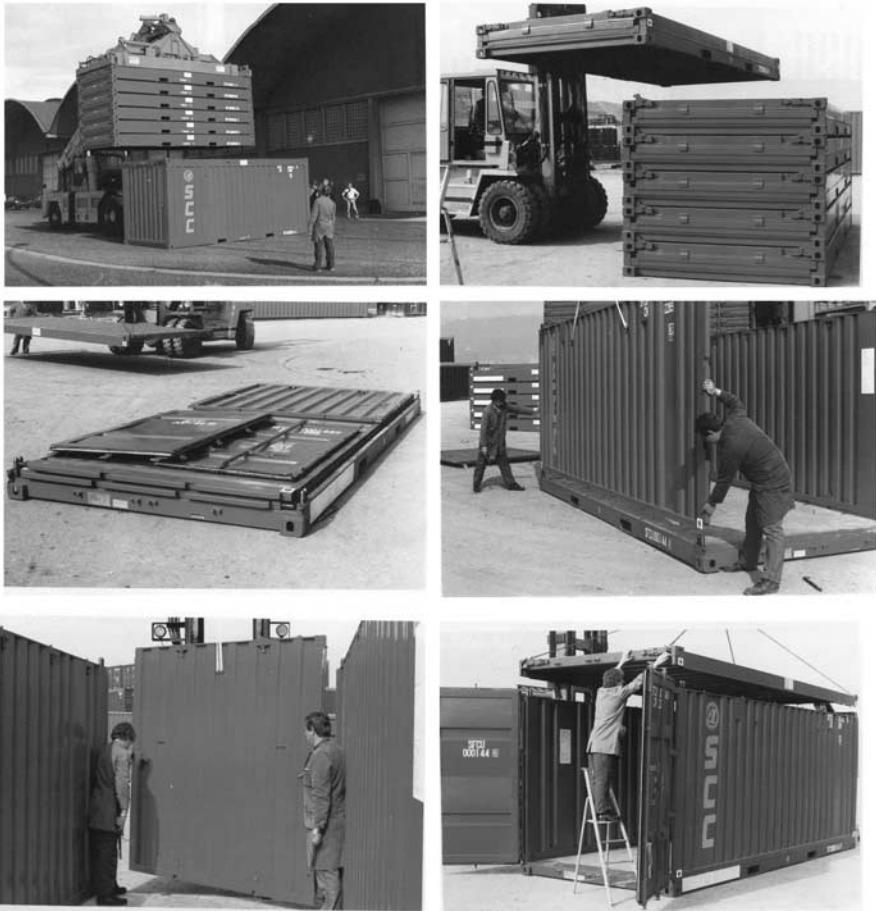
Figure 5: The folding process of the Six-In-One container
